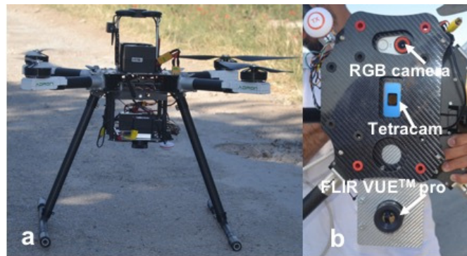
Fig. 3. Quadcopter used for the test (a); optical sensors on board (b)
